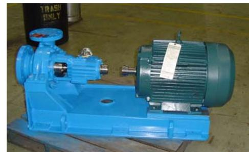
**Custom drop-in pump matched hydraulics of the existing pumps.**
